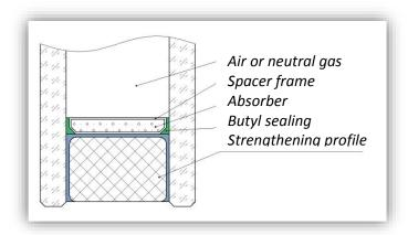
Thus, the structural strengthening of the unit stiffness is designed by modification of a typical double-glazed unit by replacing the secondary containment with tightly glued composite profile of rectangular cross section.
