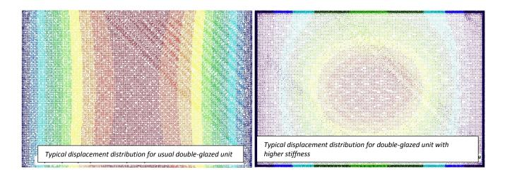
When a solid pultruded profile with section of 16x16mm and elasticity modulus of  $5*10^8$  N/m<sup>2</sup> as a stiff spacer in DGUHS is used, the following formula is applicable to calculate the thickness of the equivalent glass with accuracy of  $\pm$  8%:
